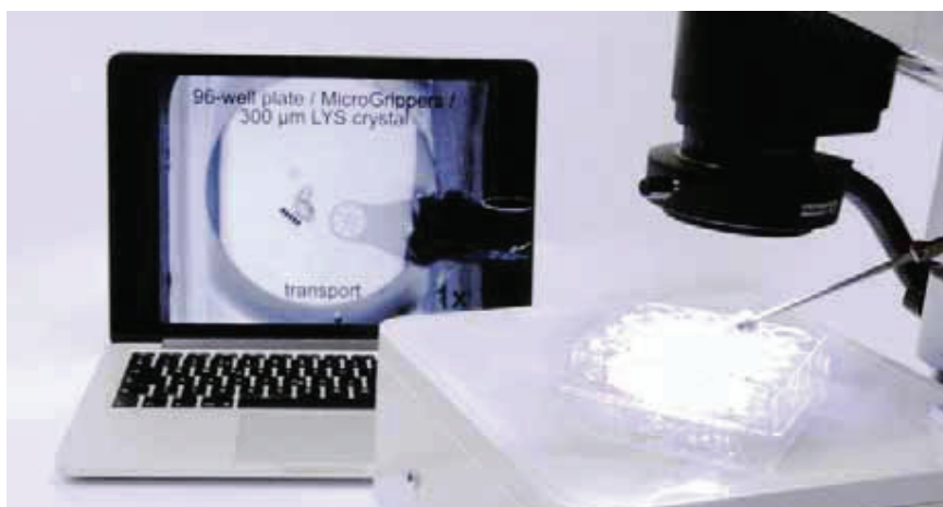
Figure 1: Protein crystallisation: RodBots are rod-shaped, magnetically responsive micro-robots (typically 50µm by 50µm by 300µm) that roll on a supporting surface and induce fluid flow in the surrounding solution. These localised flows can pick up and transport crystals and place them onto a loop or other extraction device. Manipulation is thus done in a non-contact manner and the gentle, distributed fluid forces safely deliver fragile protein crystals to their destination 2 (see www.magnebotix.com )
