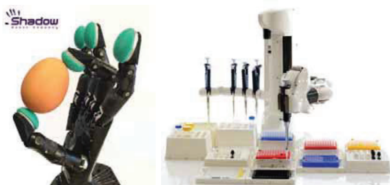
Figure 2: Some example systems: the Shadow Robot hand (left) offers the full five fingers of manipulation. The Andrews Alliance arm (right) uses standard pipettes and offers a degree of co-bot capability. While mobile robots from companies such as Adept and Bosch are now available to perform sample logistics, new humanoid robotic platforms such as the iCub could allow the next generation of lab robot to successfully operate a wider range of tools and instruments around the laboratory
